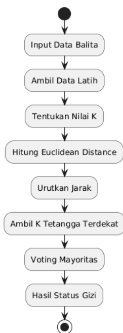
Gambar 3. Flowchart Algoritma KNN
